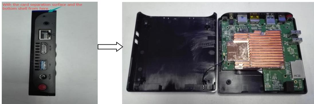
3、 Gently remove the antenna and snap motherboard screws
