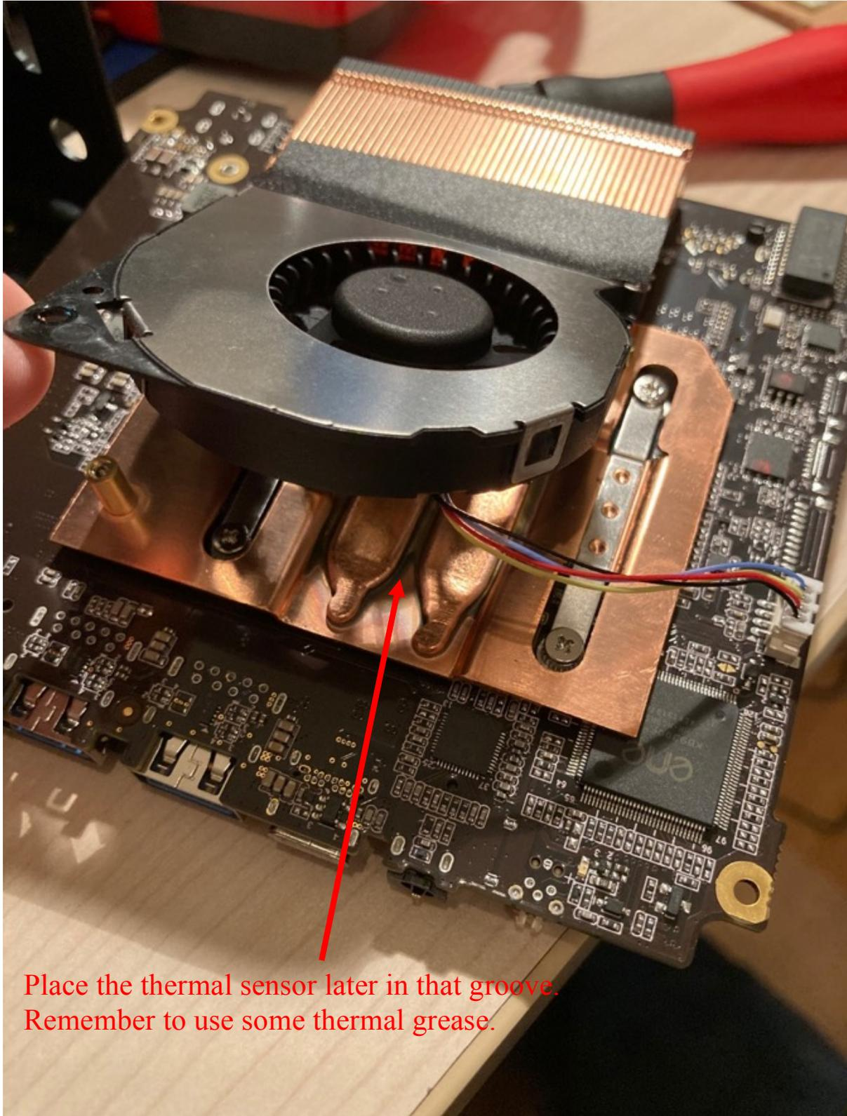
Place the thermal sensor later in that groove.
