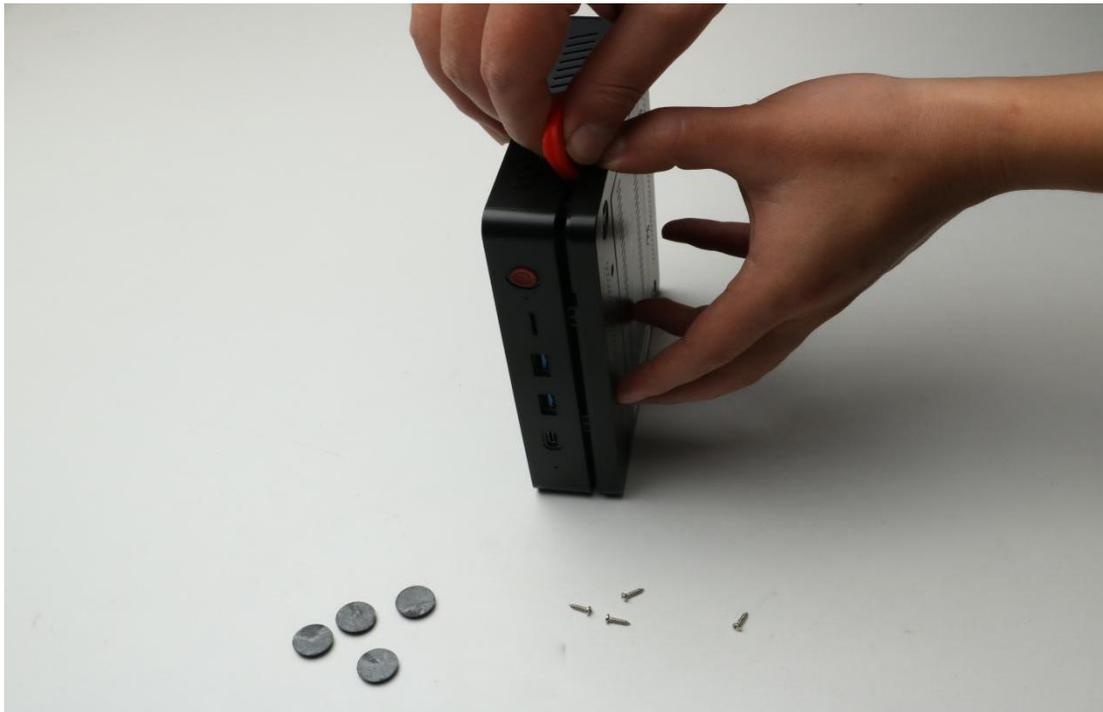
4 , Remove the two fixing screws on the motherboard
